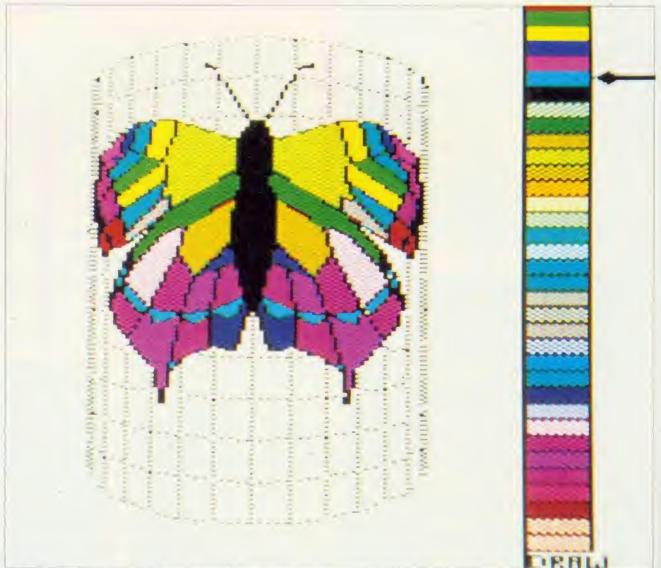
The use of colour in non-linear transformations: the start co-ordinates of the colour fill sequence have been subject to the same transformations as the points in the motif
